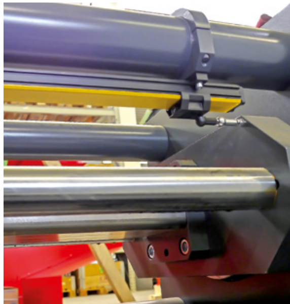
The sensor withstands vibrations and shocks of up to 200 g and supplies consistently precise measured values
